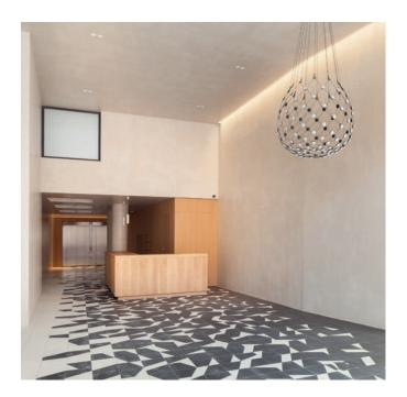
site and oak veneer door assembly, all lacquered with white Ral 9016 open-pore semi-satin paint. Walls and ceilings of plasterboard painted with Ral 7002 matt plastic paint. Lighting: Bega 22816 wall lights on doors with lighting/numbering assembly. iGuzzini Underscore Grazer Led strips in plasterboard false ceiling moulding. iGuzzini model 351 recessed luminaires with MY24 lens.
